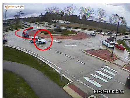
Figure 1. Still from conflict video showing vehicle cutting from the outer to inner roundabout lane
